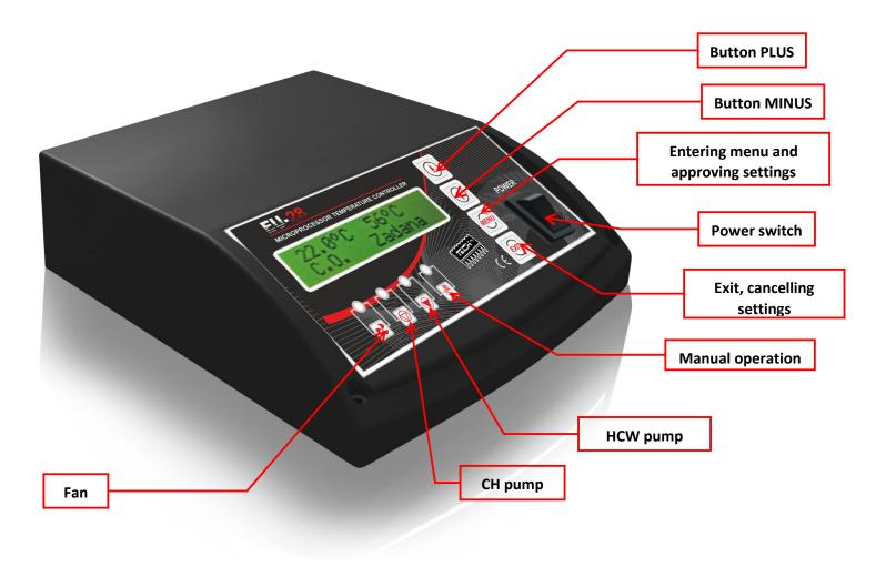
The **EU-28zPID** temperature regulator is intended for use with central heating boilers. The regulator is used for controlling the central heating water circulation pump, hot consumption water pump and blow (fan).
