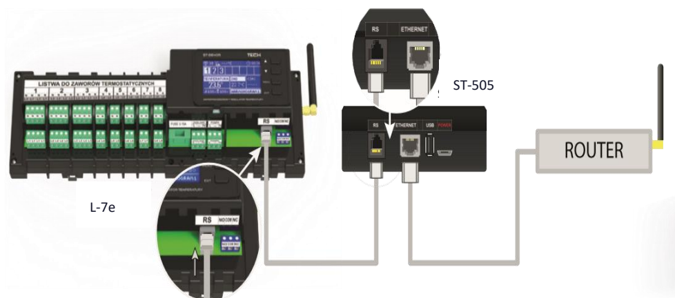
Connection diagram for ST-505 Internet module.
