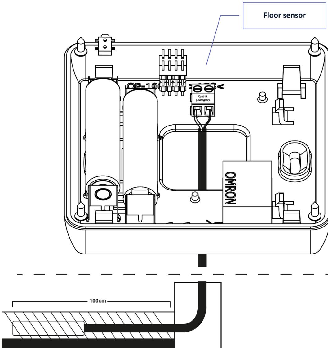
The room regulator should be connected to the heating device with a two-core cable. The cable connection between both devices is shown in the diagram below::
