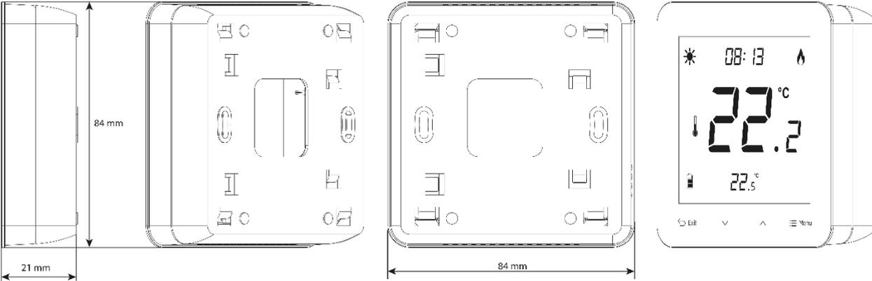
In order to mount the regulator on the wall, screw the rear cover onto the wall, insert batteries and slide the device into the cover.
