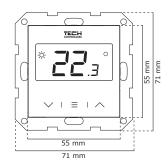
The EU-F-2z v2 regulator communicates with the heating device by means of a radio signal sent to the receiver. The receiver is connected to the heating device using a two-core cable. It communicates with the room regulator using a radio signal.
