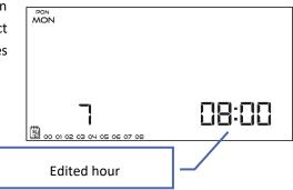
The parameters of the weekly program are displayed at the bottom of the screen: hours to which comfort temperature has been assigned are displayed whereas hours to which economical temperature has been assigned are not displayed.
